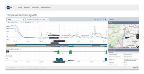
Picture caption: cargofleet 3 gives a quick overview of the fleet and individual functions - the screenshot shows the temperature profile of a refrigerated semitrailer. (Source: idem telematics GmbH)
