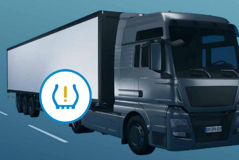
The UN ECE R 141 prescribes, among other things: If a tyre pressure loss of 20% or a malfunction occurs, the driver must receive a warning in the cab within ten minutes.
